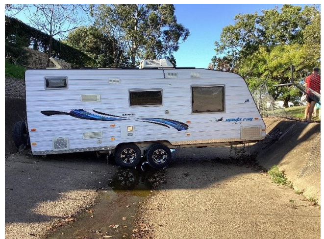
Figure 2 The outcome of an unhitched caravan without wheel chocks, roll back at Bundaberg RV Park.
